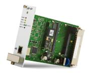
The VIP series offers multi-functional Video Image Processing modules for traffic control. VIP boards integrate automatic incident detection, data collection, recording of pre and post incident image sequences and streaming video in one board. VIP modules have been installed for road and tunnel projects all over the world.
